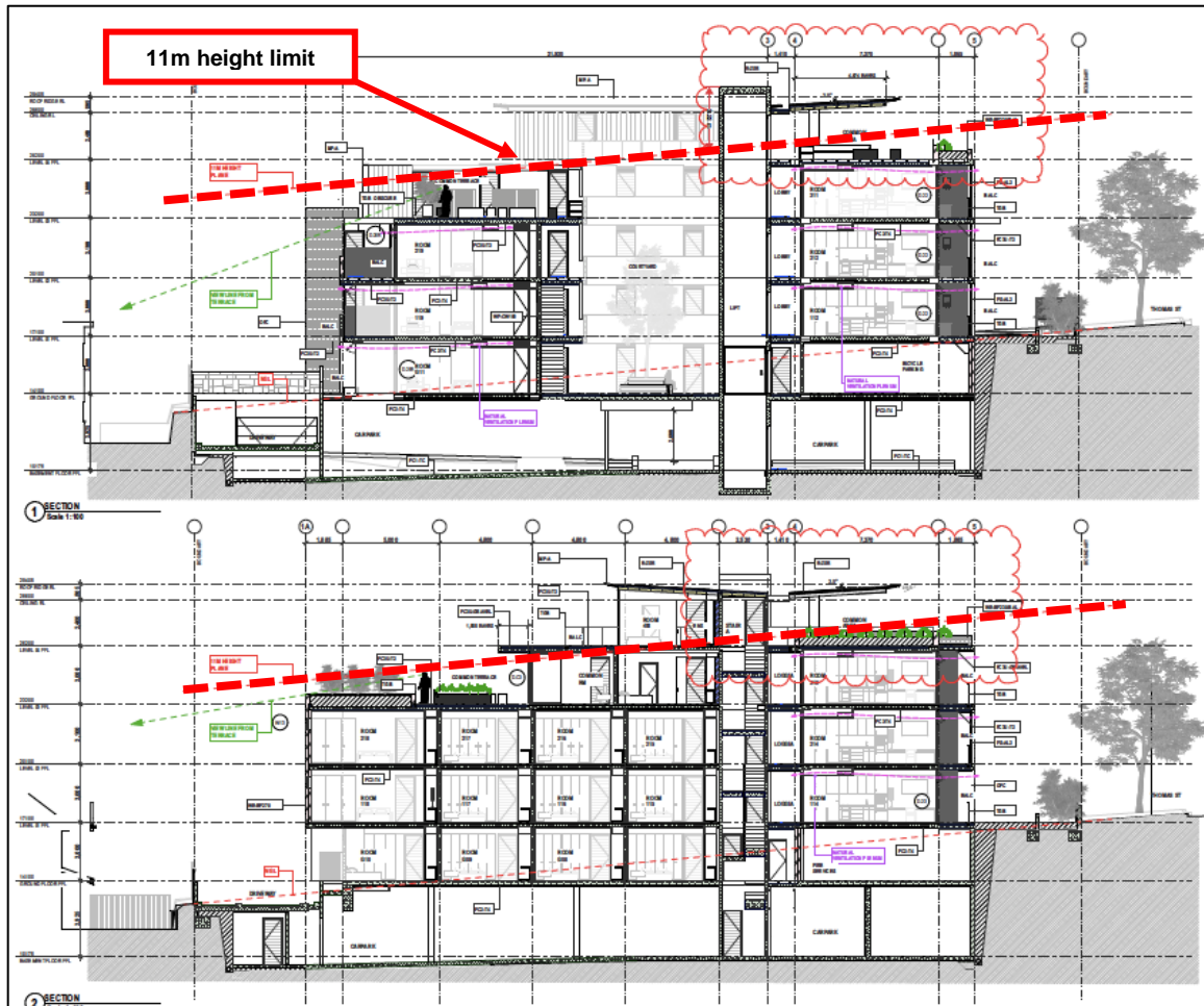
Figure 1: Section drawing extracts indicating height variation based on natural ground level ( Source: VOARC)
